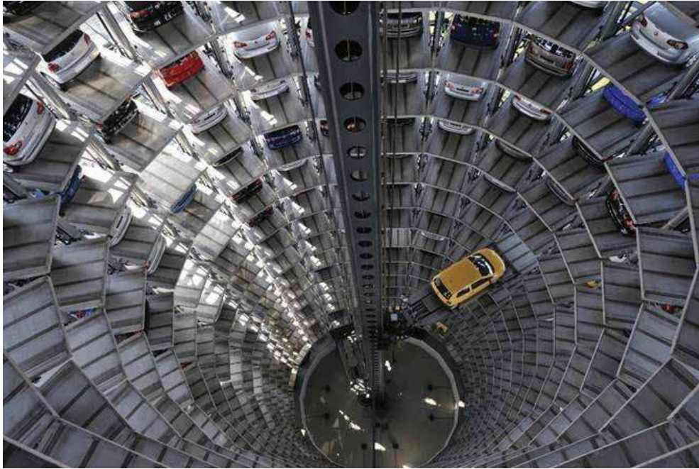
● A vehicle is lifted inside a parking tower
